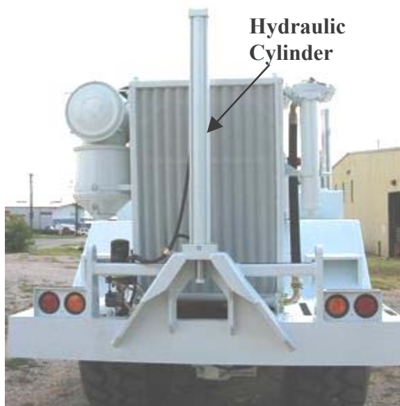
a. Hydraulic cylinder used to push (or retrieve) sensors into ground
