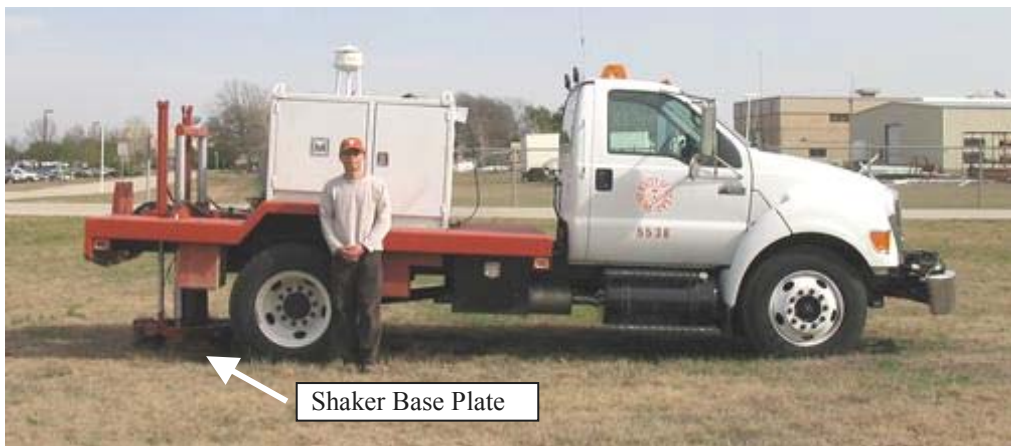
c. High-frequency, three-axis shaker called Thumper
