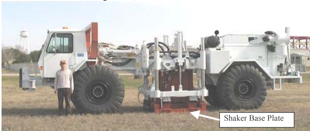
a. High-force, three-axis shaker called T-Rex
