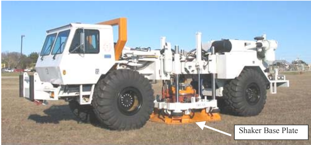
a. High-force, three-axis shaker called T-Rex
