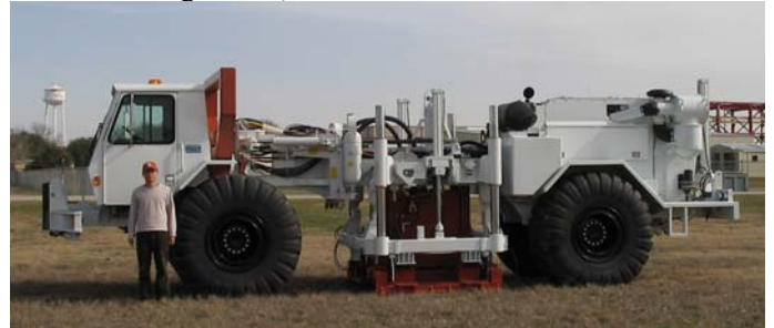
b. Low-frequency, two-axis shaker called Liquidator
