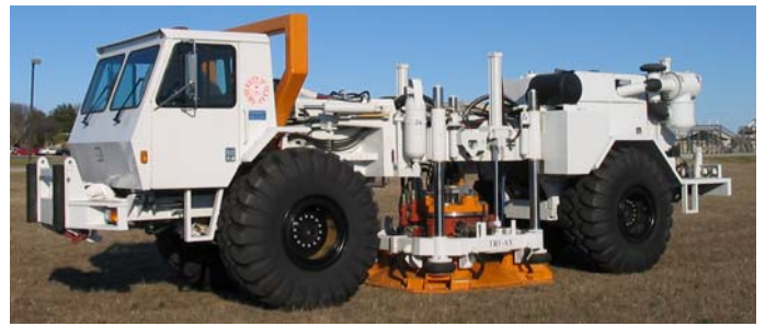
a. High-force, three-axis shaker called T-Rex
